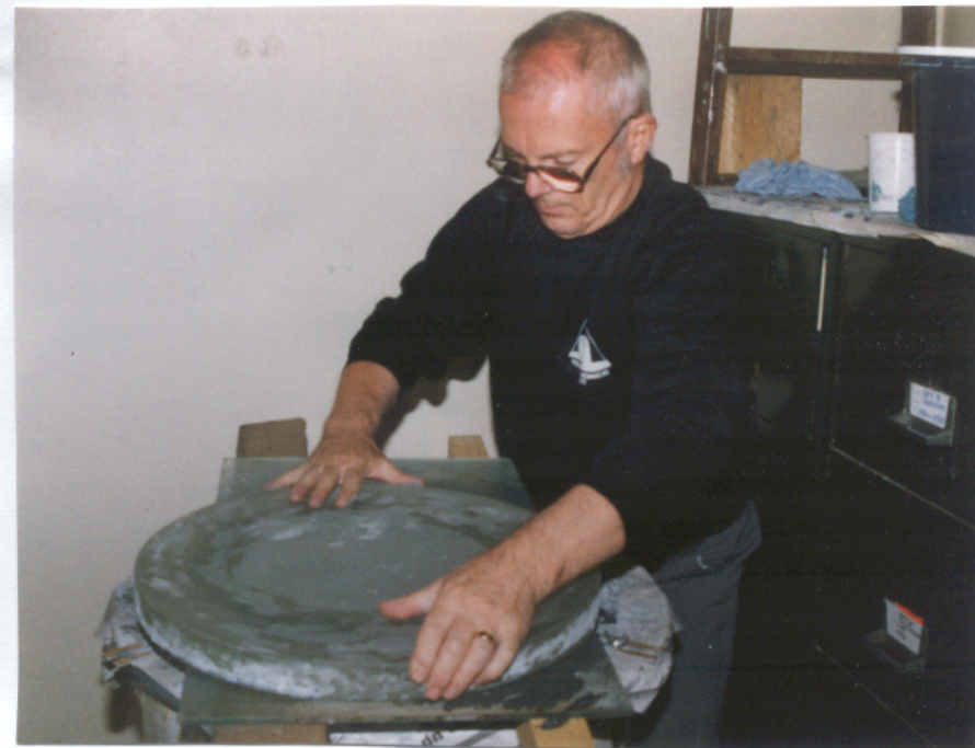
S J Robinson beginning the grinding of the rear face of the blank to achieve a flat surface Photo by Ken Goward
