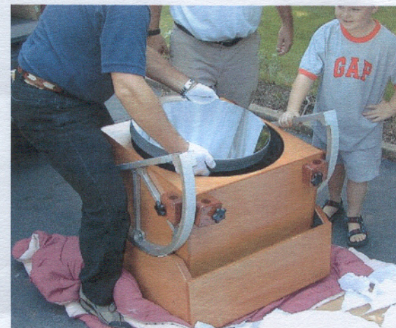
Figure 2 - Inserting Primary Mirror During Assembly
