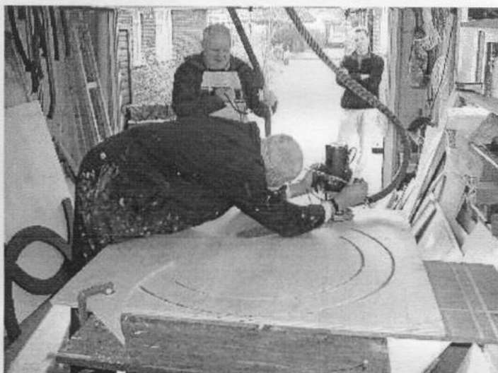
Figure 5 – Routing the plywood (side bearing)
