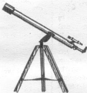
A typical small refractor on a simple stand, with a star diagonal at the eyepiece end. All diagrams by John Lewis
