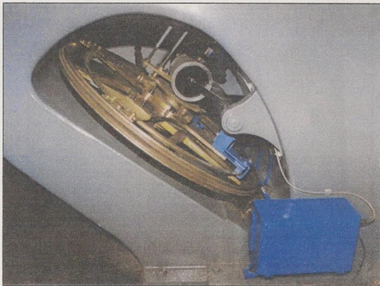
The mount of the Tomline Refractor showing the RA drive wheel and blue box containing the former electric drive.
