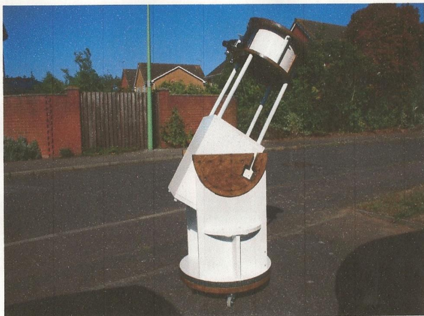
Home made 254mm 1.1 focal length Dobsonian. Built by John Wainwright.
