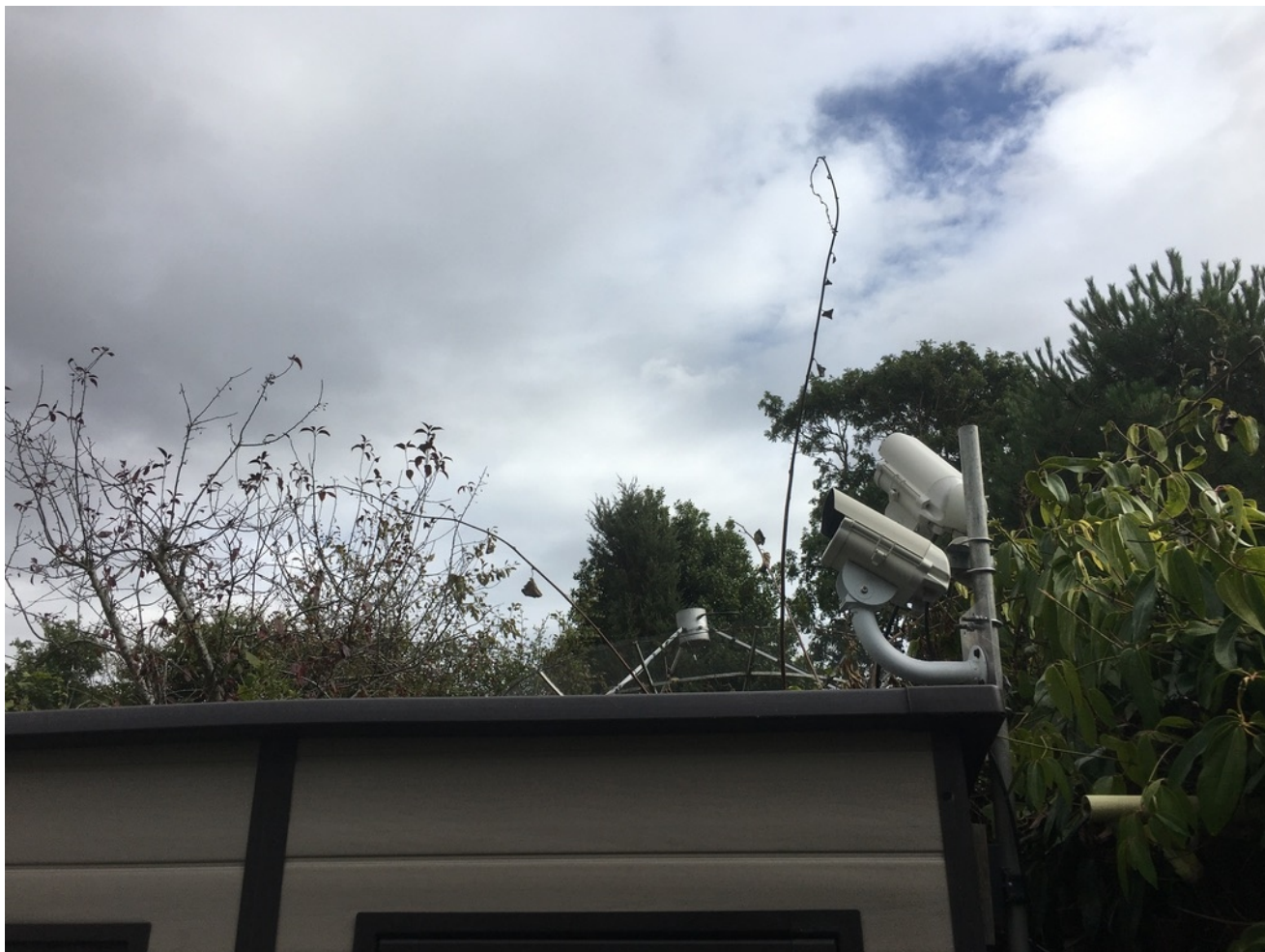
UK0007W mounted above UK0056 with 2.4m steerable dish behind the shed.
