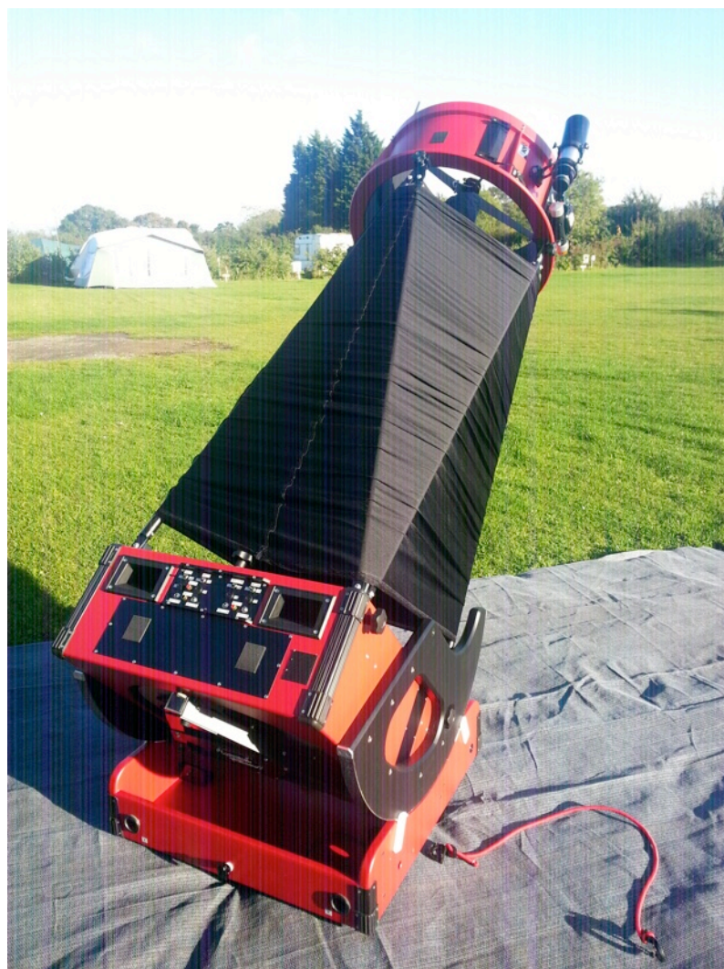
Home-made 20" go-to motorised Dobsonian
